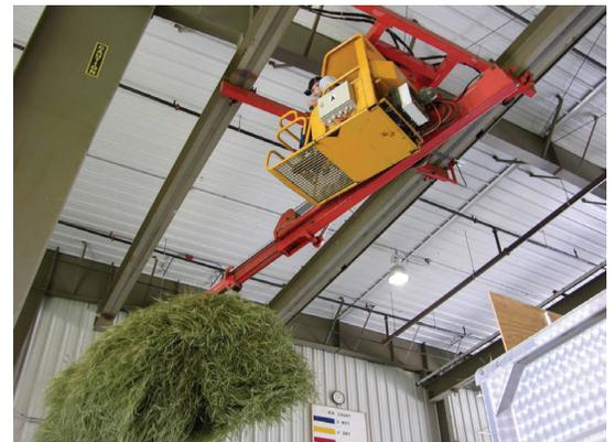
**Crane operator emptying incoming field trucks into the drying bins.**
