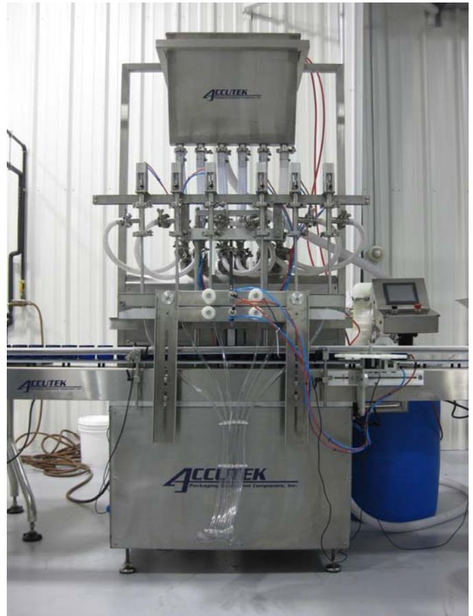
**Accutek AVF6 Automatic Piston Filler installed in our packaging line**
