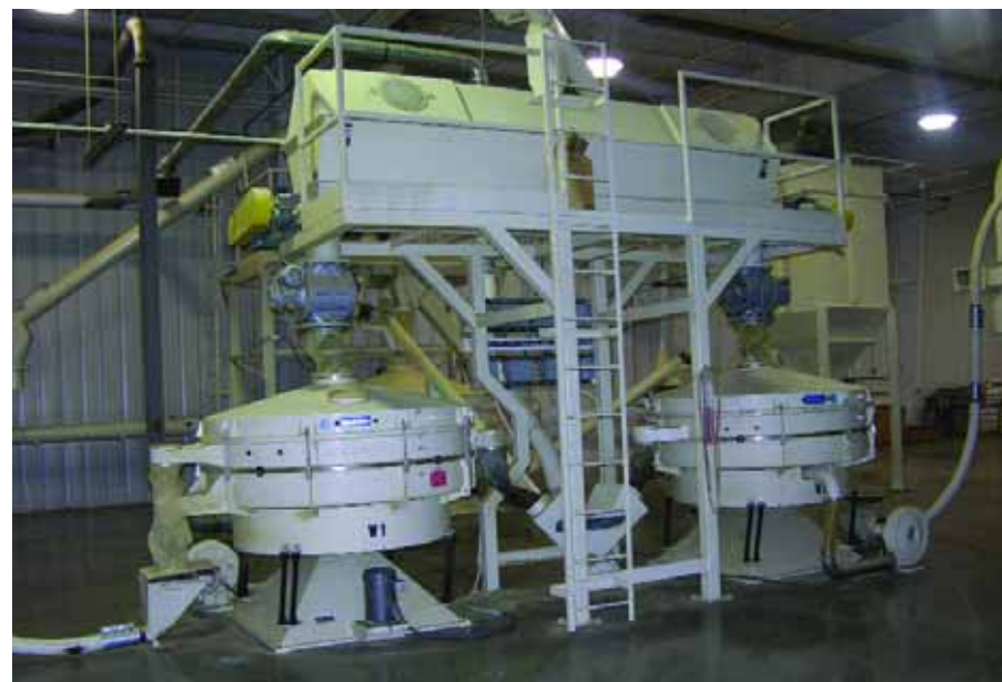
This processing area at Graminex is where the pollen is sifted out from all the other waste plant material via pneumatic conveying.
