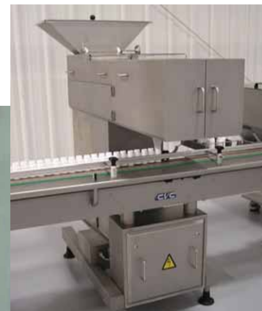
These vibratory channel plates separate tablets and capsules into 10 channels which flow into a laser counter. This provides Graminex with 100 percent accuracy. Tablets are then counted (seen above) and bottled.
