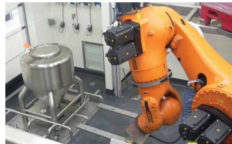
A KUKA robot removes bins from the press when they are full of processed tablets.
